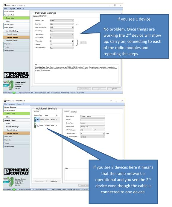
Step 4: Make Sure the RS485 settings match the settings for the Energy Meters and The Gateway.
